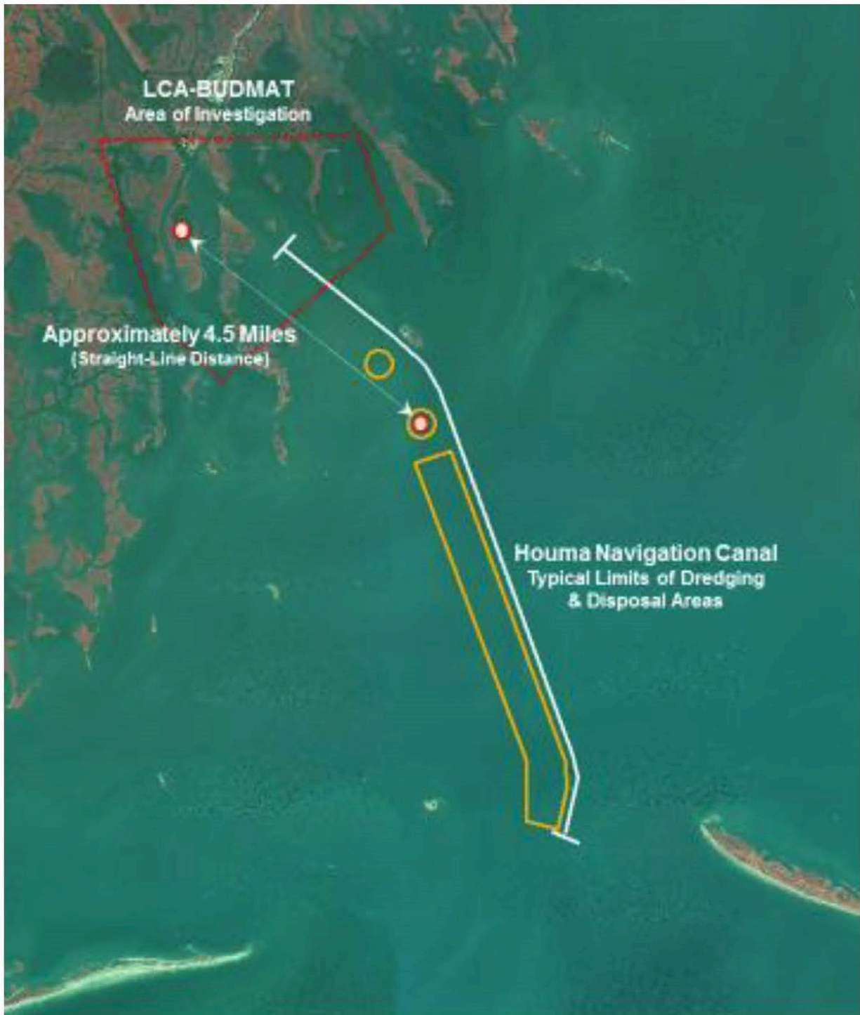
Figure 3: Approximate location of the Houma Navigation Canal (Terrebonne Bay Reach) and the LCA Budmat area (red polygon) with typical limits of dredging (white line) and Federal Standard open-water disposal areas (yellow-orange) used during routine channel maintenance.
